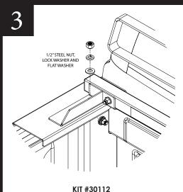
Fasten the RealTruck Backrack Assembly to the Stake pocket bolt as shown.
