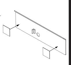
Apply single sided adhesive pads to this side of spacer. Apply RealTruck Backrack decal \*\*Can also be applied as last step to ensure facing outward\*\*
