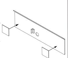
Apply single sided adhesive pads to this side of spacer.
