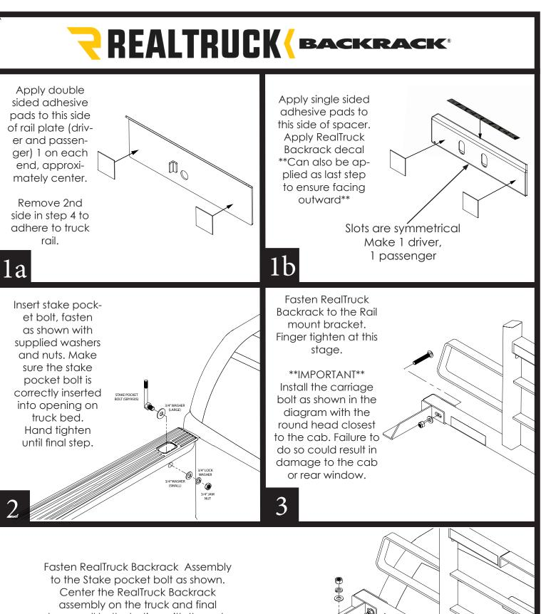
torque all bolts starting with the nuts on the inside of the truck bed, then the rail mount bracket and finally the main RealTruck Backrack carriage bolt.
