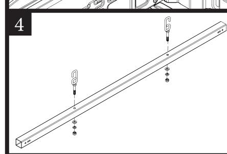
Install tie downs to center holes as shown in diagram using nuts and washers.
